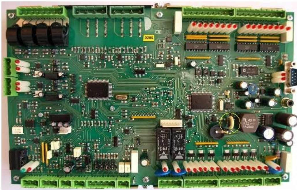
Image 3.10 IS-CU: Battery position on the PCB
