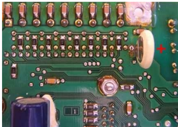
Image 3.6 IG/IS-NT: Battery position on the PCB
