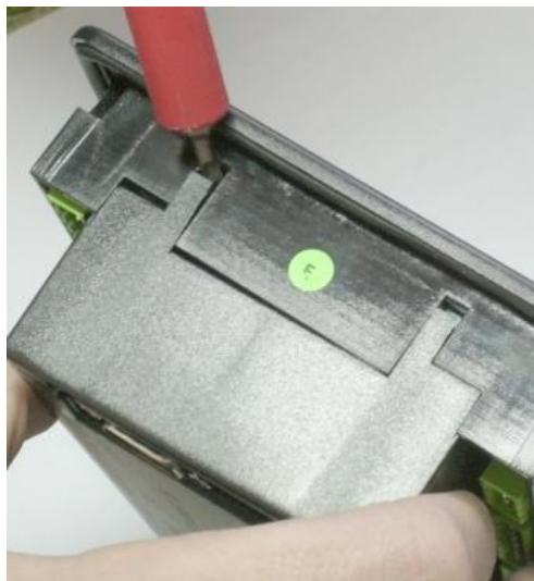
Image 3.12 Removing the rear cover
