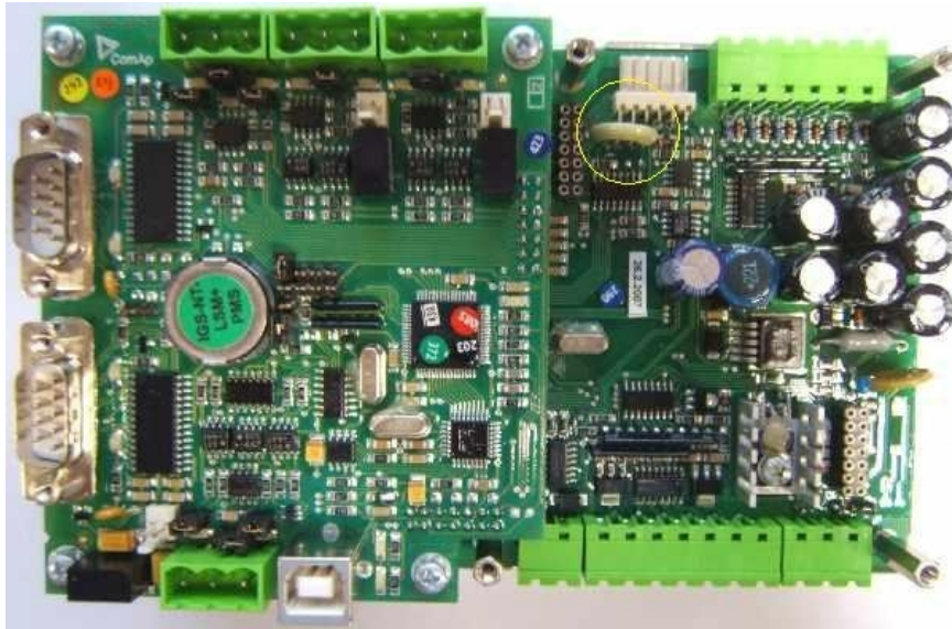
Image 3.2 IG/IS-NT: Battery position on the PCB
