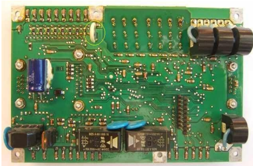
Image 3.5 IG-CU: Battery position on the PCB
