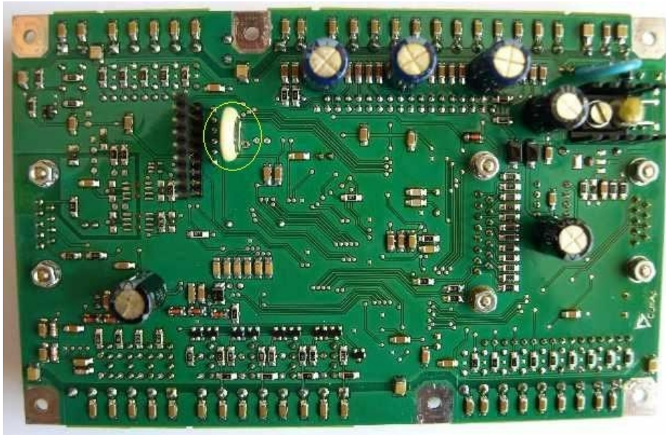
Image 3.8 ID-DCU: Battery position on the PCB
